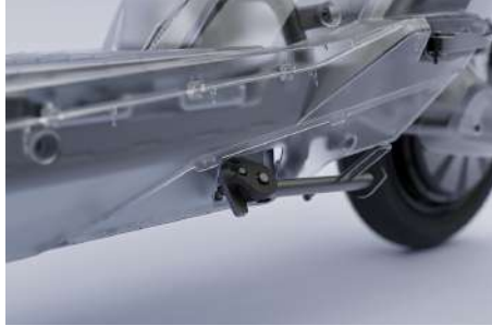
Integrated Side Stand Sensor.
